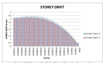
Graph 5.2 Storey Drift in X and Y with shear wall
