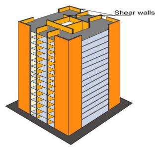
Fig 1.5 Building with Shear wall
